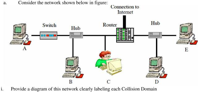
Domain 1: A - Switch Port for A Domain 2: Switch Port for Hub I; B;Hub I;C; Router Port to C Domain 3: Router Port for Hub II; B;Hub II ;D; E Domain 4: Router Port for Internet Feed
