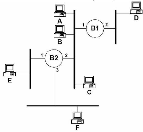
Show the forwarding table in each of the bridges after the following transmissions (which occur in the given order), assuming each table starts out empty:
